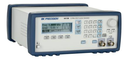
Models 4007B and 4013B are versatile DDS (direct digital synthesis) sweep function generators with high signal precision and stability. These instruments generate sine and square waveforms up to 7 MHz or 12 MHz, including triangle waveforms up to 1 MHz. Both models provide variable output voltages from 0 to 10 Vpp into 50 ohms or up to 20 Vpp into open circuit. A continuously variable DC offset allows the output to be injected directly into circuits at the correct bias level.
